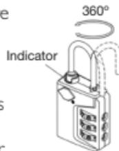
To return the red collar to its original hidden position, simply turn the dials to your combination, pull up the shackle and turn it 360° counterclockwise until you hear the sound of a click, or insert a small pin-like device (paperclip, pen point, etc.) into the small hole that is located on the side of the lock housing, on the opposite end of the dials.
