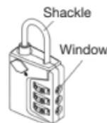
**Step 2:** Pull up the shackle and turn 90° counterclockwise to align the nub on the shackle with the notch on the lock body.
