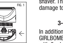
2. Hold shaver handle and lift head up from the back (see FIG.1), then press foil frame release buttons on each side and lift up (the cutter will now be in view). Be careful not to push on the foils. They are delicate and can easily be damaged.
