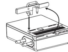
**Australia, China, Fiji, and New Zealand** – Gently press the button and completely slide to the left for USA/AUST plugs as shown. Make sure the contacts are rotated to the "I" position. Pull out the insulated ground pin and insert it into the corresponding position as shown.
